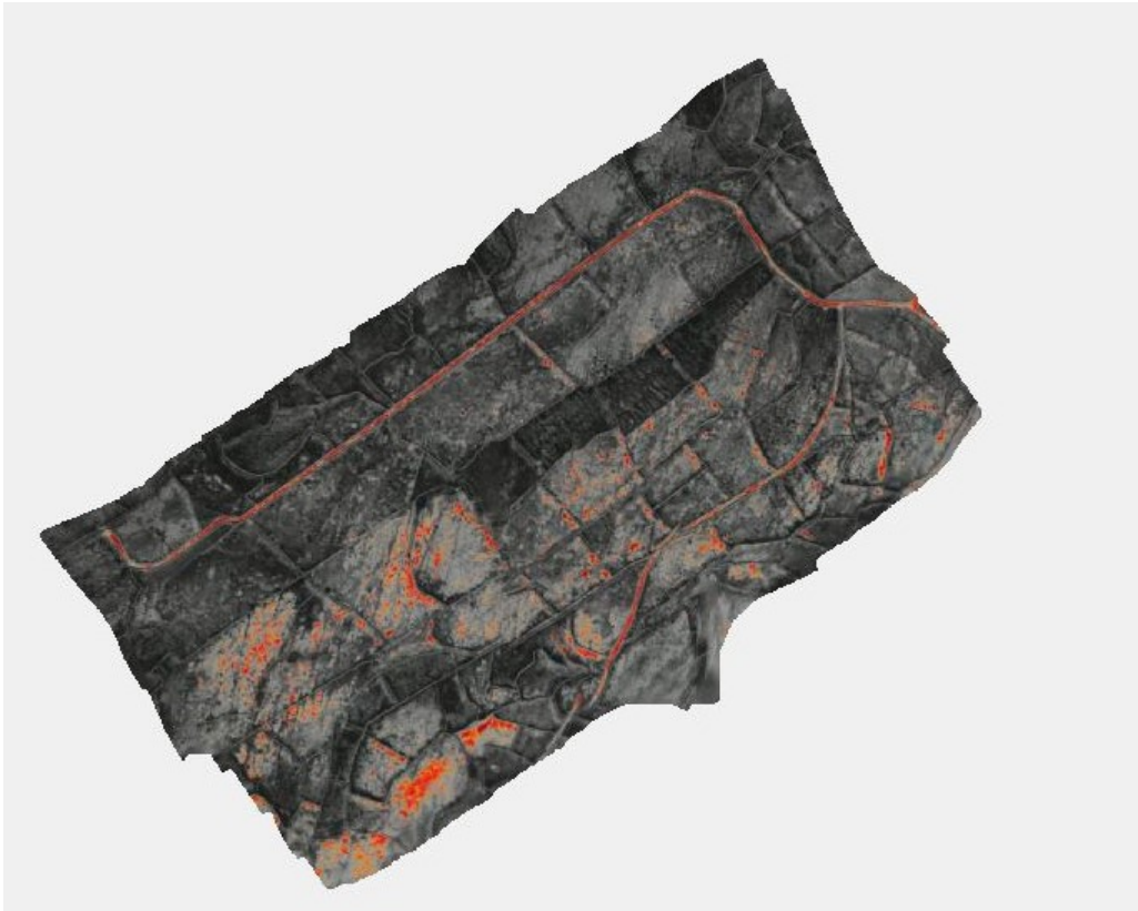
Image 2: Site 1, Mavic Duo (thermal) tied down with recorded GCP's
