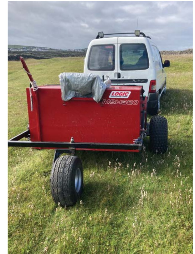
Fig.9 Gathering wildflower seed, machine drawn brush harvester
